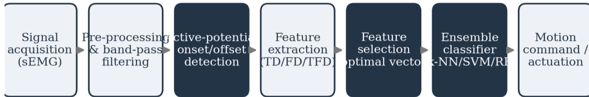
Real-time hand-movement recognition pipeline
